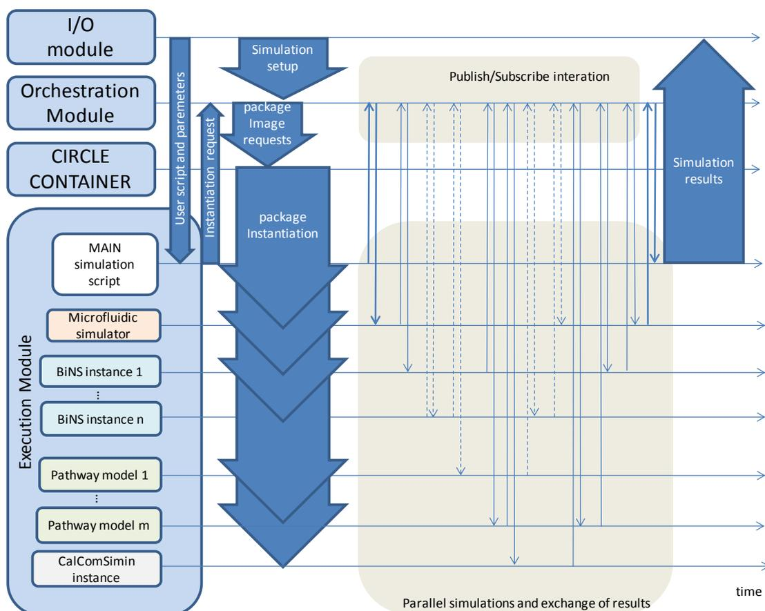
Figure 3. Interactions between the entities of the CIRCLE MolCom Toolbox.
